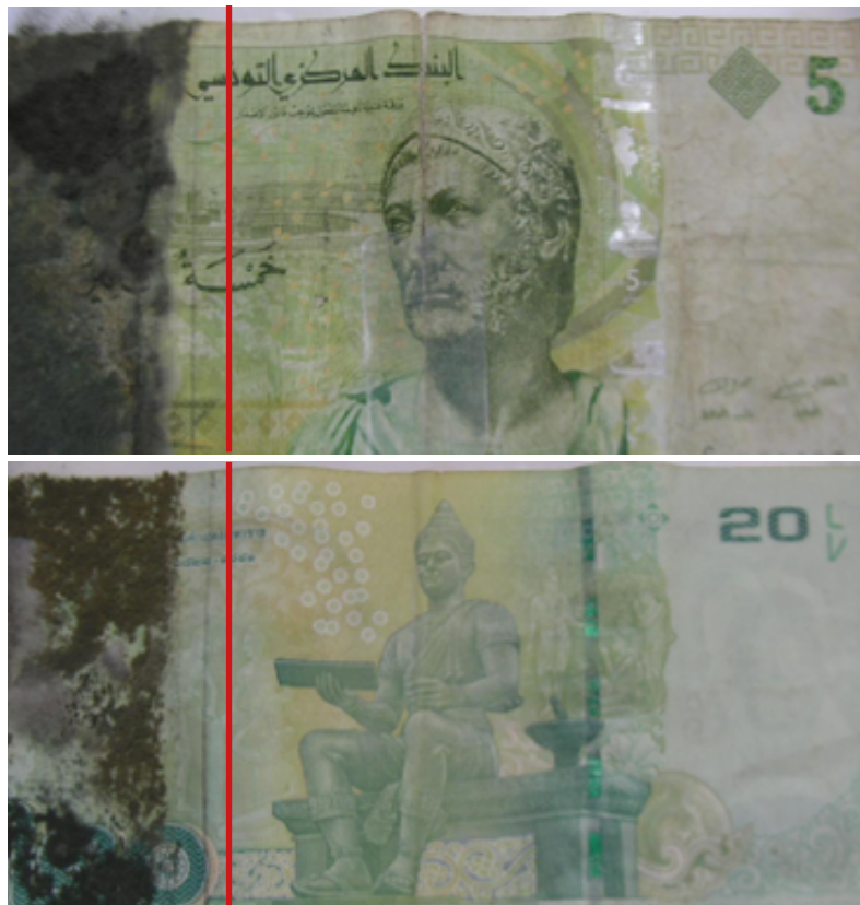
To the left of the red line is the mould on banknotes that have not been treated with Intace Protect® after six day's exposure to humidity, whilst to the right are the same banknotes to which Intace Protect® has been applied.
